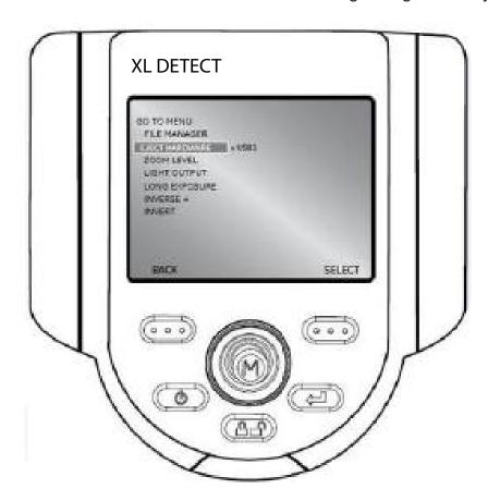
Note: Always use EJECT HARDWARE before removing a USB thumb drive to prevent loss of data.
