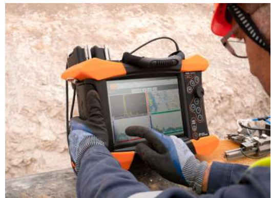
In-field inspection using M2M Gekko
