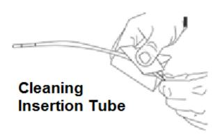
3 – Clean the rest of the probe, including insertion tube and fiberoptic connector. Use a soft cloth dampened with glass cleaner or 70% alcohol-to-water solution.
