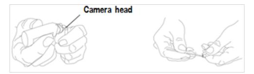
**2** – Clean the probe tip, including the lens on the camera head. Use glass cleaner or 70% alcohol-to-water solution and a pointed cotton swab.
