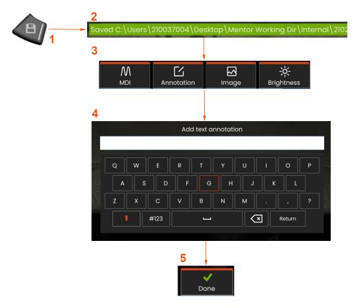
Image files can be stored in the Mentor Flex or a detachable device. The **Quick-Save** feature stores a file with a default name and file type in a default directory Alternatively, use the **Save Options Menu**.
