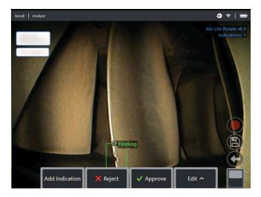
4. Now save image containing inferences or alternatively cycle through the bounding boxes to 'accept', 'reject' and alter any classification(s) as desired.
