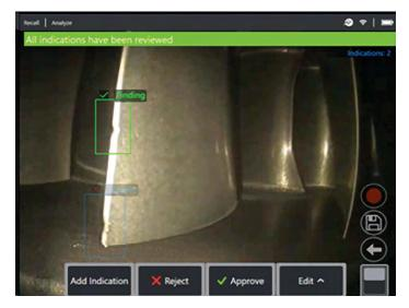
Once the image is saved and then subsequently recalled, only the 'accepted' bounding box(es) will be immediately visible. The remaining bounding boxes remain present but hidden from view.
