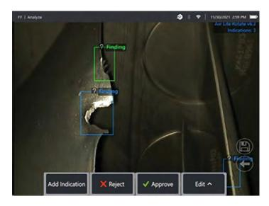
Initiate 'Freeze Frame' to activate Aiir Lite - Rotate analytic.
