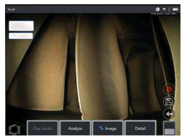
Tap the softkey page button to present the second row of softkeys. Select 'Analyze' softkey in order to process the image for indications.
