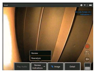
The handset overwrites any prior assignments e.g. acceptance or rejections and displays the output from the activated analytic.
