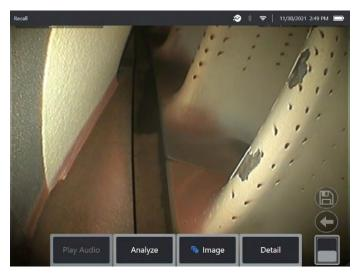
2. Tap the softkey page button to present the second row of softkeys. Select 'Analyze'. softkey in order to process the image for indications.
