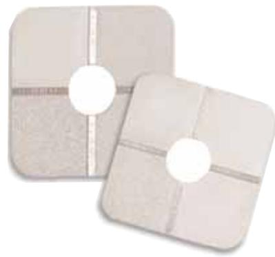
Each comparator has four segment profiles for comparison:
