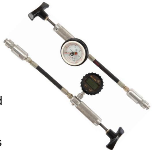
When the stress exceeds the adhesion of the coating, the dolly and coating detach from the substrate. The maximum value of hydraulic pressure during the test is recorded and is equivalent to the adhesion of the coating to the substrate.
